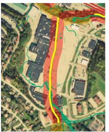
Figure 6: Example of Riparian Buffer analysis that highlights stream course through parking lot. Yellow line indicates the likely stream course through culverts underground.
