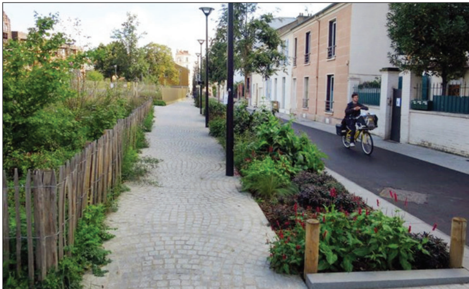
A ‘green’ alley in Philadelphia, with streetside rain garden.
