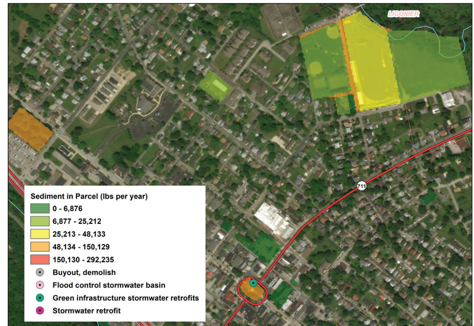
Enlarged plan of Ligonier, Loyalhanna Watershed Area of Interest indicating impacts and opportunities for BMPs
